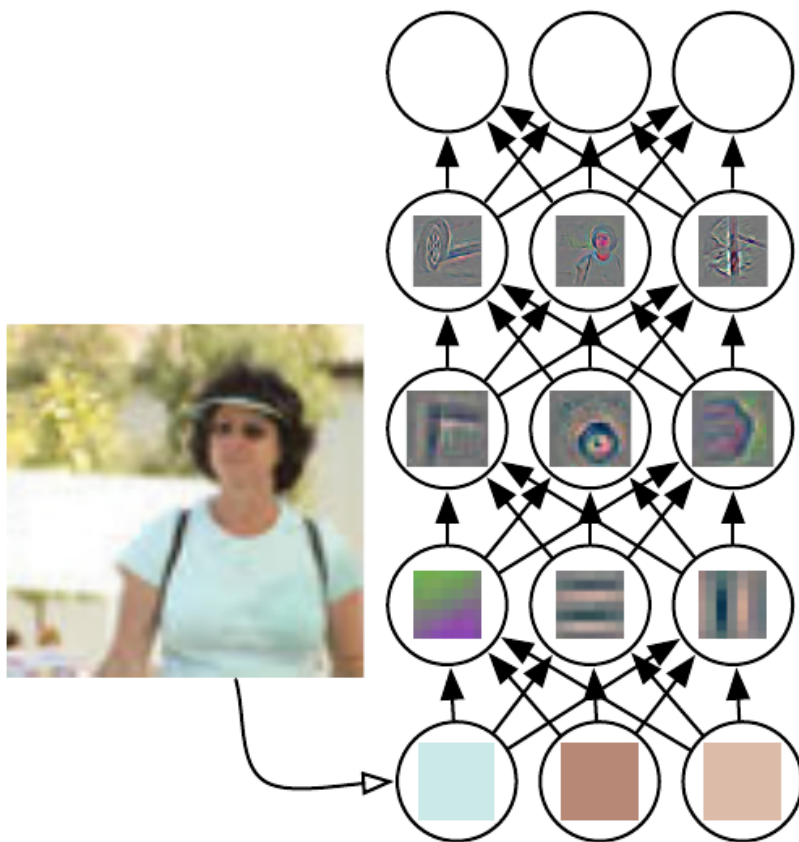
Figure 1.2: Illustration of a deep learning model. It is difficult for a computer to understand the meaning of raw sensory input data, such as this image represented as a collection of pixel values. The function mapping from a set of pixels to an object identity is very complicated. Learning or evaluating this mapping seems insurmountable if tackled directly. Deep learning resolves this difficulty by breaking the desired complicated mapping into a series of nested simple mappings, each described by a different layer of the model. The input is presented at the input , so named because it contains the variables that we are able to observe. Then a series of hidden layers extracts increasingly abstract features from the image. These layers are called “hidden” because their values are not given in the data; instead the model must determine which concepts are useful for explaining the relationships in the observed data. The images here are visualizations of the kind of feature represented by each hidden unit. Given the pixels, the first layer can easily identify edges, by comparing the brightness of neighboring pixels. Given the first hidden layer’s description of the edges, the second hidden layer can easily search for corners and extended contours, which are recognizable as collections of edges. Given the second hidden layer’s description of the image in terms of corners and contours, the third hidden layer can detect entire parts of specific objects, by finding specific collections of contours and corners. Finally, this description of the image in terms of the object parts it contains can be used to recognize the objects present in the image. Images reproduced with permission from Zeiler and Fergus (2014) .
